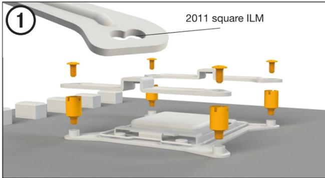
**Assembly of the cooler mounting frame**
