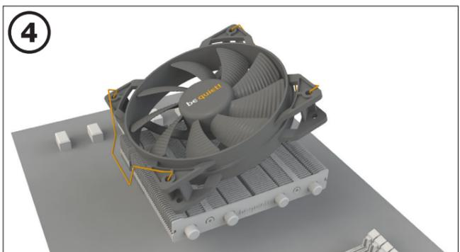
Fasten the 120mm fan onto the cooler unit using fan clips. Connect the fan to the motherboard's PWM signal.
