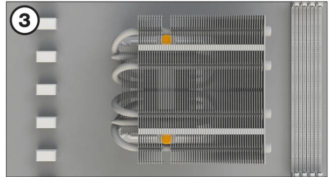
Position the cooler mounting bridge centrally on the cooler. Insert the mounting bridge fastening screws from above into the cooler mounting bridge and then screw these alternately tight. You can use any cross-tip screwdriver for this.
