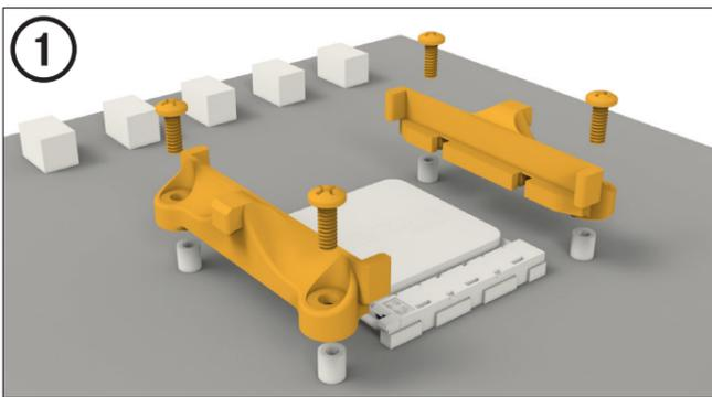
**Assembly of the cooler mounting frame**
