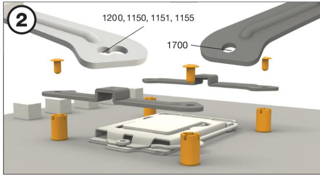
**Installation of the mounting brackets**
