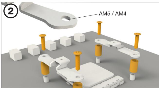
Place the four AMD spacer nuts onto the backplate bolts protruding through the front side and affix both short AMD mounting brackets with the AMD backplate screws.
