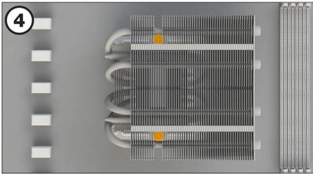
Position the cooler mounting bridge centrally on the cooler. Insert the mounting bridge fastening screws from above into the cooler mounting bridge and then screw these alternately tight. You can use any cross-tip screwdriver for this.
